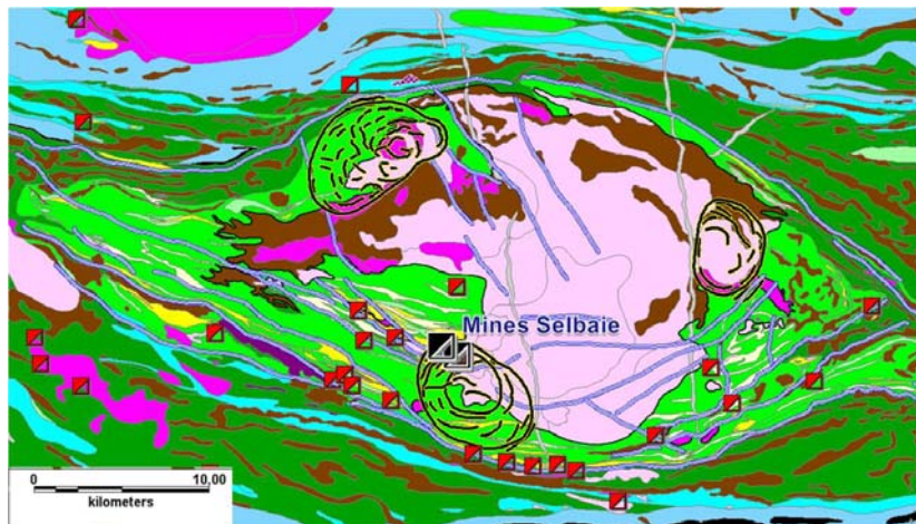
New geological map of the Selbaie mining camp showing synvolcanic faults and structures of the inferred calderas. The Brouillan intrusive complex at the centre is surrounded by Brouillan andesites (pale green) and felsic volcanics (pale yellow). The eye is surrounded by the Enjalran-Bapst Group (basalts).
