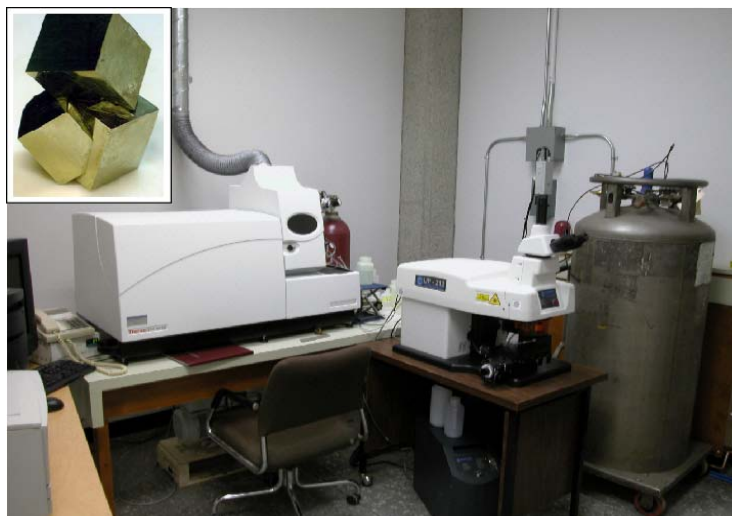
A new machine at the cutting edge of technology, the LA-ICP-MS, is used to determine trace elements contained in pyrite.
