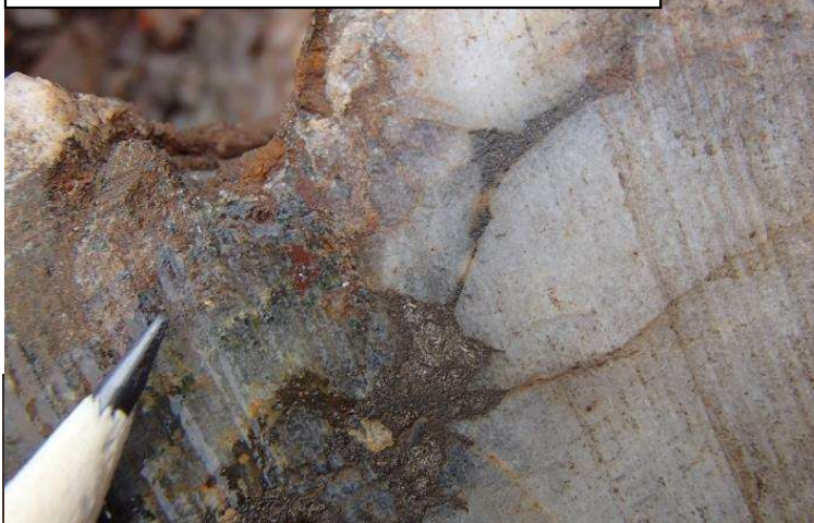
FAU2015TR015-R4 7.9m Visible gold in wallrock of a Qtz-Po-Ank-Chl vein
